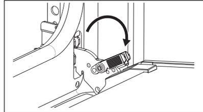
3. Close the oven door halfway to the first opening position. Then lift and pull to remove the door from its seat.
