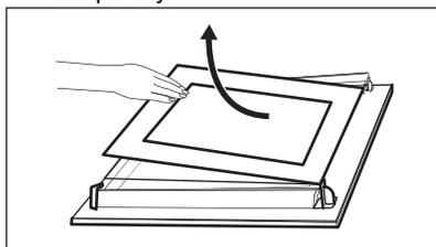
8. Clean the glass panels with water and soap. Dry the glass panels carefully. Do not clean the glass panels in the dishwasher.
