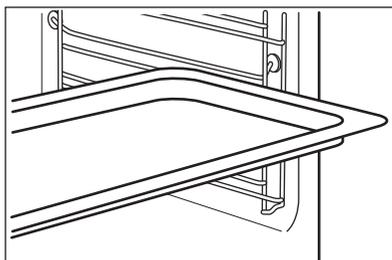
Push the tray between the guide bars of the shelf support. Place the baking tray with the slope towards the back of the oven interior.
